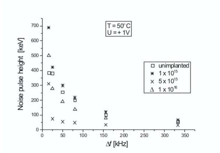
Fig. 2. Frequency noise level of three implanted and one unimplanted sample at 50°C
