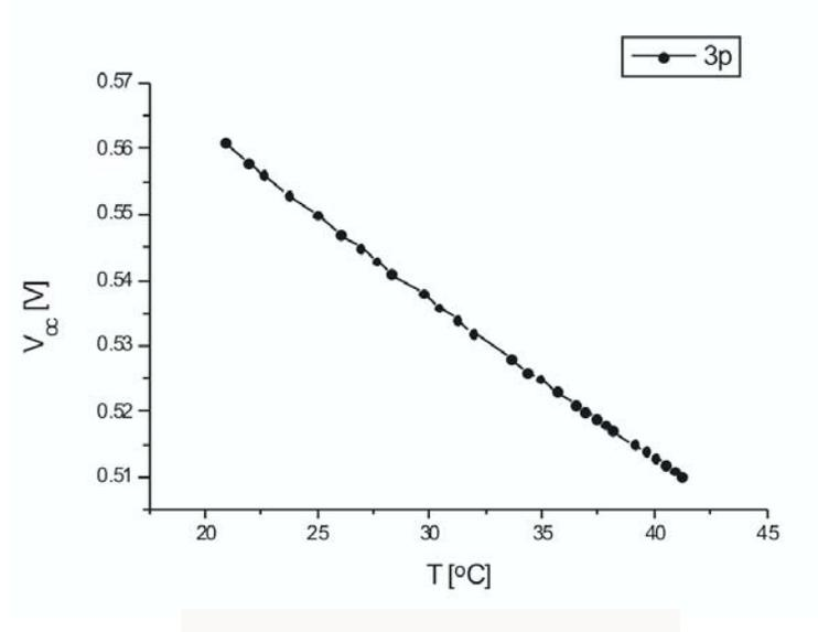
Fig. 3. Temperature dependence of open circuit voltage  $V_{oc}$ .
