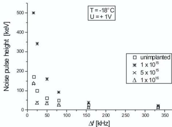
Fig. 1. Frequency noise level of three implanted and one unimplanted sample at  $-18^{\circ}\text{C}$
