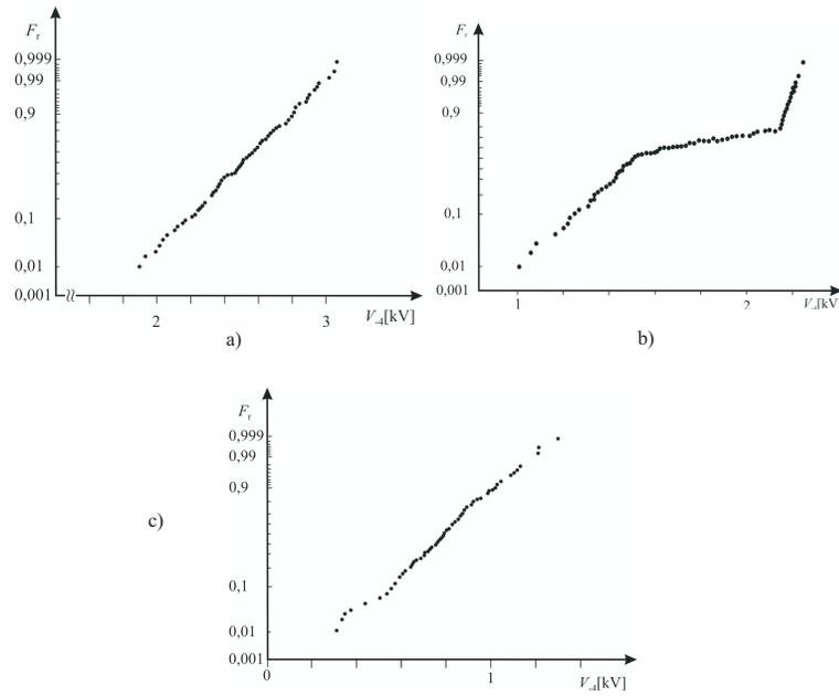
Fig. 10. Emission characteristics presented on the Weibull probability plotting paper at pressures a)  $10^{-6}$  mbar, b)  $10^{-2}$  mbar, and c)  $10^{-1}$  mbar, for the inter-electrode gap of 0.1 mm.
