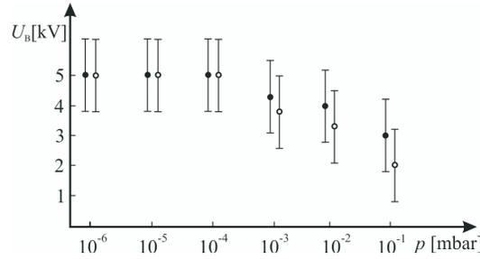
Fig. 5. Dependence of dc ( $\circ$ ) and impulse ( $\bullet$ ) breakdown voltage mean values and the corresponding standard deviations on pressure of the residual gas ( $\text{SF}_6$ ), at the inter-electrode gap of 0.1 mm.
