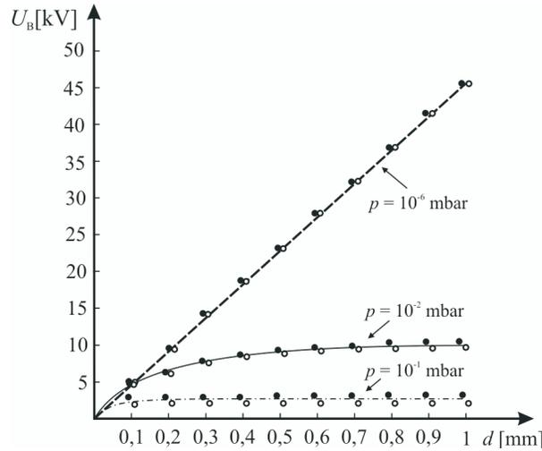
Fig. 4. Rate of breakdown voltage rise as a function of the inter-electrode gap (impulse (o) and dc (•) breakdown voltage mean values).
