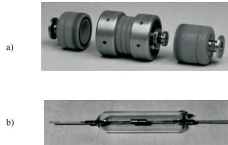
Fig. 1. a) Specially constructed chamber used for investigations in the pressure range from 1 bar to  $10^{-1}$  mbar. b) Vacuum diodes used for investigations in the pressure range from  $10^{-1}$  mbar to  $10^{-6}$  mbar.
