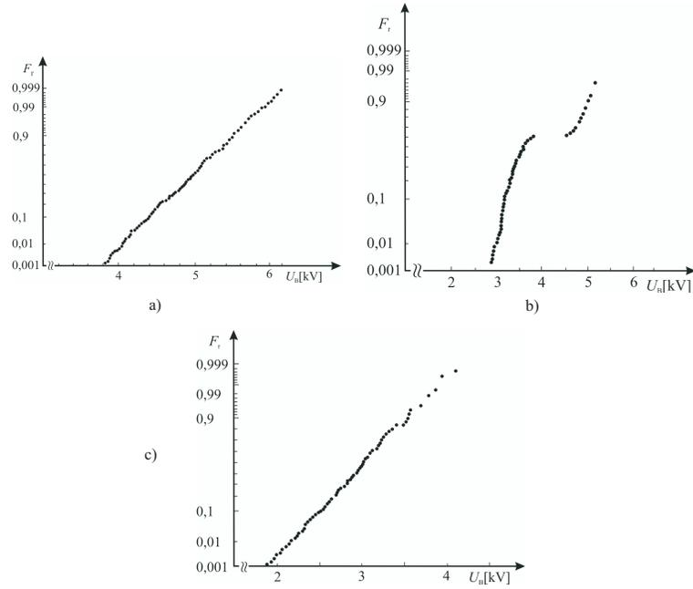
Fig. 9. Impulse breakdown voltage presented on the Weibull probability plotting paper at pressures: a)  $10^{-4}$  mbar, b)  $10^{-2}$  mbar, and c)  $10^{-1}$  mbar, for the inter-electrode gap of 0.1 mm.
