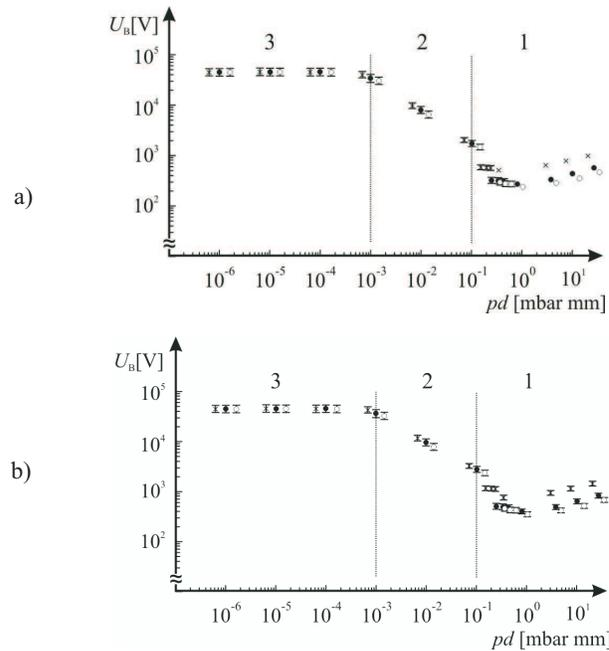
Fig. 2. a) Dependence of dc breakdown voltage mean value on the  $pd$  product (pressure  $\times$  inter-electrode gap), with the gas type as a parameter (o – Ar, • – N<sub>2</sub>, x – SF<sub>6</sub>), at the inter-electrode gap of 1 mm. b) Dependence of impulse breakdown voltage mean value on the  $pd$  product (pressure  $\times$  inter-electrode gap), with the gas type as a parameter (o – Ar, • – N<sub>2</sub>, x – SF<sub>6</sub>), at the inter-electrode gap of 1 mm.
