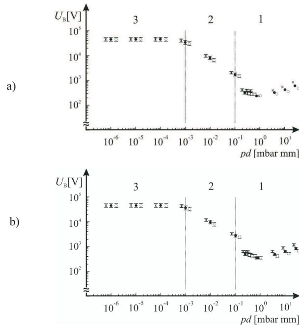
Fig. 3. a) Dependence of dc breakdown voltage mean value on the  $pd$  product, with the electrode material as a parameter ( $\circ$  - elektron,  $\bullet$  - aluminium,  $\times$  - tungsten), at the inter-electrode gap of 1 mm. b) Dependence of impulse breakdown voltage mean value on the  $pd$  product, with the electrode material as a parameter ( $\circ$  - elektron,  $\bullet$  - aluminium,  $\times$  - tungsten), at the inter-electrode gap of 1 mm.
