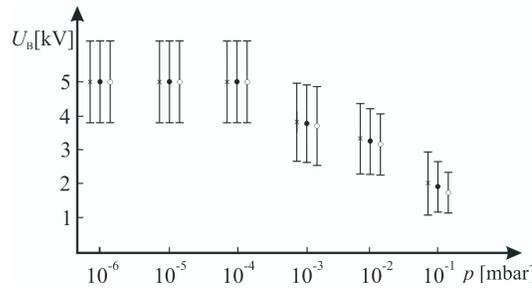
Fig. 6. Dependence of the dc breakdown voltage mean value on pressure, with the residual gas type as a parameter ( $\circ$  - Ar,  $\bullet$  - N2,  $\times$  -  $\text{SF}_6$ ), at the inter-electrode gap of 0.1 mm.
