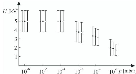
Fig. 7. Dependence of the dc breakdown voltage mean value on pressure, with the electrode material as a parameter ( $\circ$  - elektron,  $\bullet$  - aluminium,  $\times$  - tungsten), at the inter-electrode gap of 0.1 mm.
