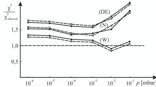
Fig. 8. Dependence of the  $\chi^2$  test variable (in relative units with relation to the maximum allowed value of the test variable, with a 5% level of significance) for random variables dc (---) and impulse (—) breakdown voltage on pressure, at the inter-electrode gap of 1 mm; (DE) double exponential distribution, (N) Normal distribution, (W) Weibull distribution.
