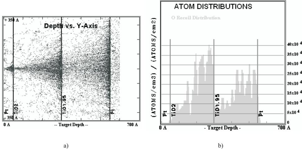
Fig. 3. Simulation results for a 10 keV carbon ion beam (100 ions) incident perpendicularly on a stacked Pt – TiO<sub>2</sub> – TiO<sub>2-x</sub>–Pt structure, with the total thickness of 60 nm. a) Ion tracks. b) Distribution of displaced oxygen atoms. Target depth axis is in units of angstrom.
