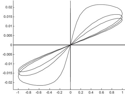
Fig. 4. Current-voltage curves of a titanium dioxide memristor, plotted for three different values of the stoichiometric region resistance:  $R_{OFF} = 18k\Omega, 16k\Omega,$  and  $14k\Omega$ . The applied sinusoidal voltage and all other parameters are the same as for Fig. 1. The decrease in  $R_{OFF}$  is caused by radiation induced emergence of oxygen vacancies in the stoichiometric  $TiO_2$  region.
