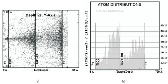
Fig. 2. Simulation results for a 10 keV proton beam (1000 protons) incident perpendicularly on a Pt-TiO<sub>2</sub>-TiO<sub>2-x</sub>-Pt stack, with the total thickness of 60 nm. a) Particle and ion tracks. b) Distribution of displaced oxygen atoms. Target depth axis is in units of angstrom.
